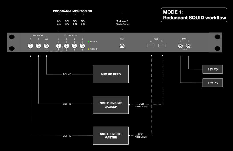
When working with a SQUID workflow and its corresponding Backup, each SQUID Engine sends its real-time status (Keep-Alive) via a USB connection to the Changeover, and this serves as an additional analysis variable for automatic switching.
